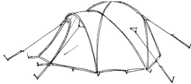
A modern geodesic nylon tent of 5 pole design
